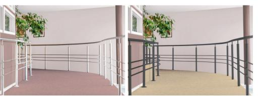
Color on handrails, carpets and pillars should contrast with the wall color with at least a minimum difference of 30 points of Light Reflectance Value. The LRV expresses the percentage of light that is reflected from a surface. To improve safety, it's important areas differentiate from each other. Color is an easy way to do this.
