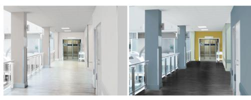
Lack of color contrast between the critical surfaces; walls, floor and doors can make it more difficult for those with visual impairments to navigate unfamiliar spaces. Add accents to make sure users can find their way, using color as signage with the right contrast improves navigation.
